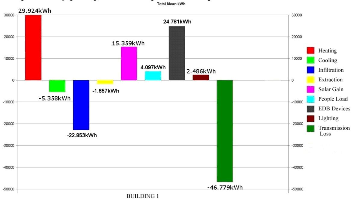
The graph above shows reference heat balance in the Supervisor's Dwelling. The heat balance is based on the future interior layout with the future people loads, where the temperature is kept at a Class C level via cooling.
