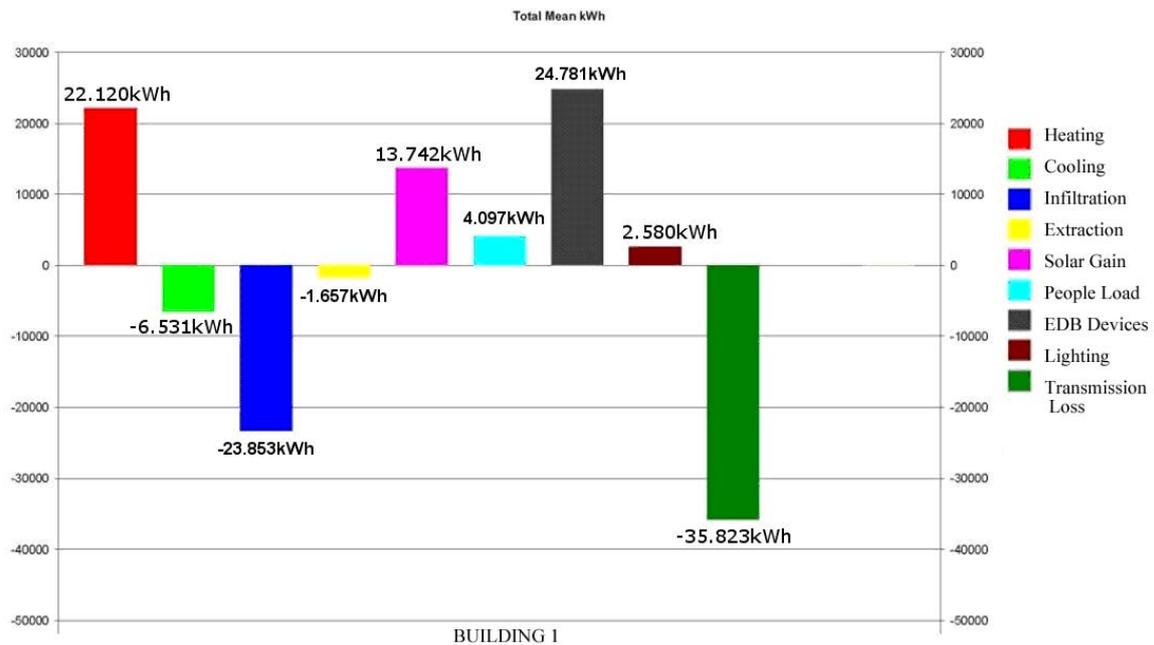
The graph above shows a breakdown of the energy use in the Supervisor's Dwelling, where the existing secondary glazing is changed to energy saving glazing. The thermal internal climate is maintained via cooling at the same level as the above reference building.
