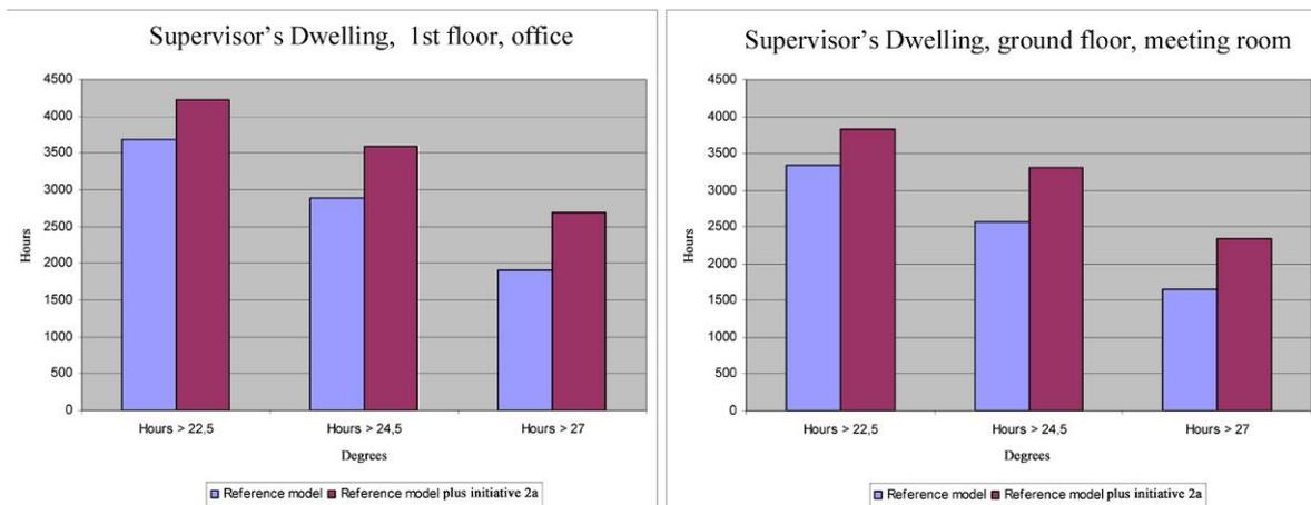
The graphs above show the number of hours where the temperature is over a specified temperature in, respectively, the first floor office and the ground floor meeting room.
