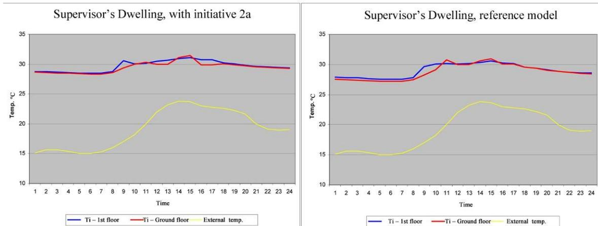
The graph to the right shows the thermal internal climate in the Supervisor's Dwelling on a summers day. The graph to the left shows the thermal internal climate on the same day with initiative 2a included in the calculation.
