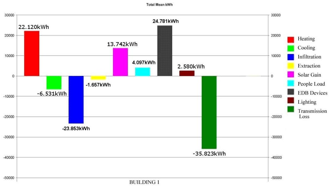
The graph above shows a breakdown of the energy use in the Supervisor's Dwelling, where the existing secondary glazing is changed to energy saving glazing. The thermal internal climate is maintained via cooling at the same level as the above reference building.
